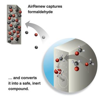
AirRenew drywall products, when used as part of a residential Indoor Air Quality design, reduce the amount of formaldehyde present in the home. This first-of-its-kind, patent-pending wallboard actively cleans air by permanently removing formaldehyde, the most common VOC<sup>2</sup> found in indoor air.
