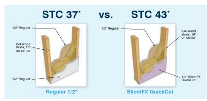
with fiberglass insulation
